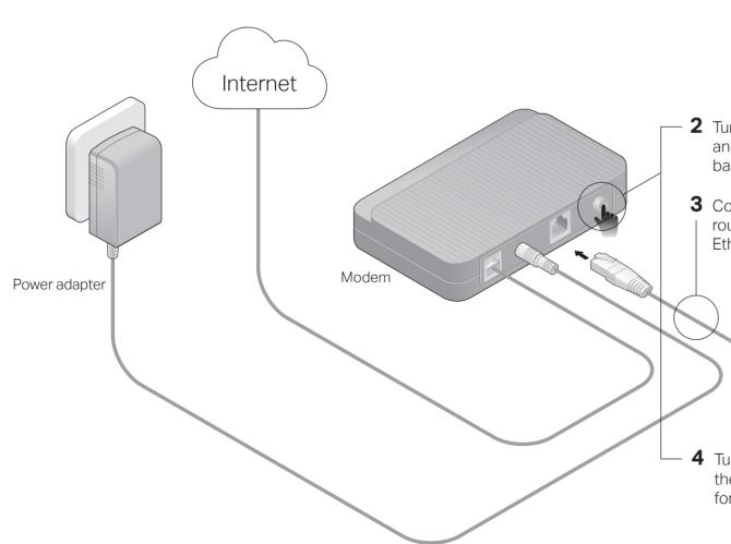
2 Turn off the modem, and remove the backup battery if it has one.
